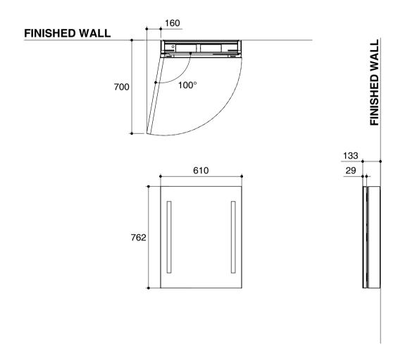
Cut-out dimensions for recess-mount installation
